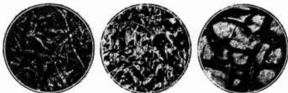
Fig. 1. Micro photos showing the surface of ink-coated, pencil-coated, and fully impregnated grid leak paper, enlarged 200 times
